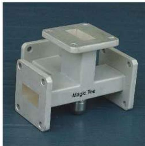
If another arm is added either to T-junction, then hybrid T-junction, is symmetrical about an imaginary plane bisecting arm3&4 and has very useful property. Magic Tee may be used in front end of the microwave receiver. The basic property in that arm3 and 4 are both connecting to
